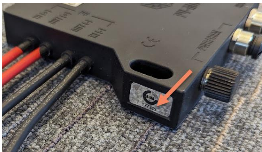
Figure 3: Modbus address is equal to the last 2 digits of the serial number. In this case '85'
